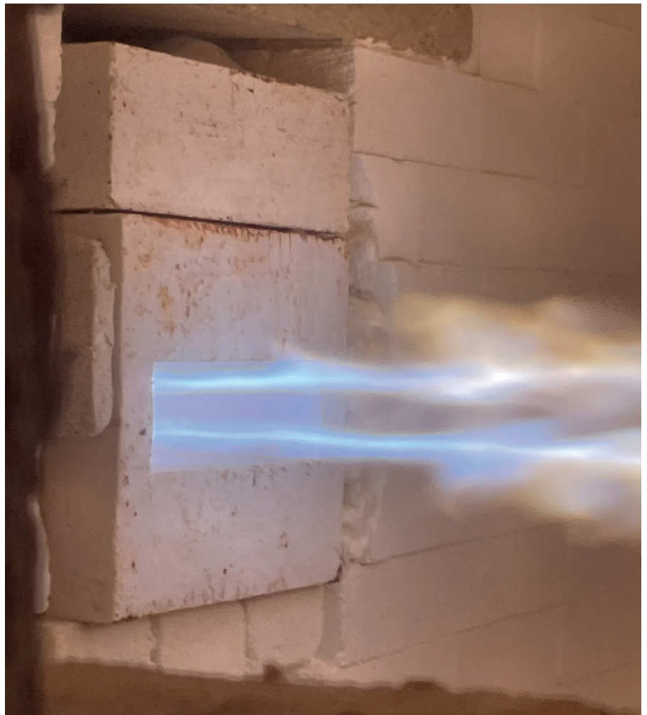
▲ Pic 2. A view of the hydrogen flat flame in the Selas testing-lab furnace.
